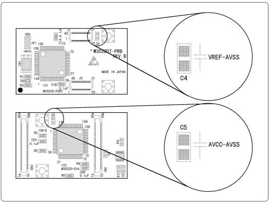
Figure 3.2 Foot patterns of A-D conversion bypass capacitor
